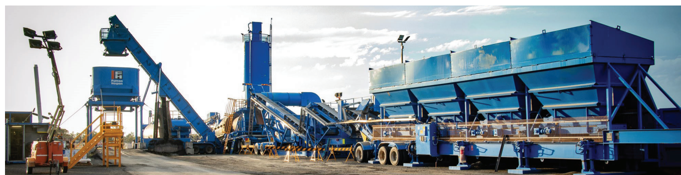
Roma Airport runway (North to South) (above). Mobile asphalt batching plant at the Roma Airport for the runway overlay project (below).
